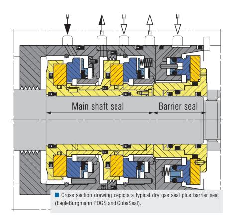
of contact between the rotating ring and stationary seal face during irregular operations such as axial vibrations or micromovements of the compressor shaft.
